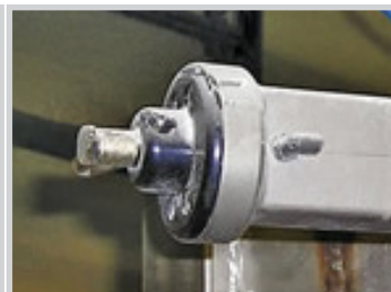
MARTIN® PKL® Interval Impactor on spout.
