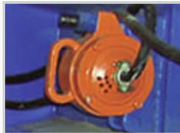
VIBROTOR™ Vibrators used on concrete form.
