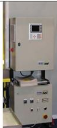
Control unit with 4 converters: 15.7"x23.6"x31.4" (WxHxD)
